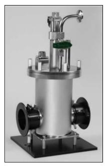
Cryostat 190 is designed to control the temperature accurately with accurate flow control of cooling nitrogen by mass flow controller and control of the heater which is kept around the sample holder. This system can be installed with FT-IR of many types and other spectrometer. This System includes Cryostat, 10L liquid nitrogen dewar, diaphragm pump (For Liquid Nitrogen flow), temperature controller and KBr windows.
